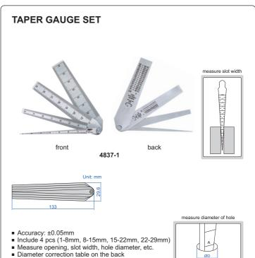
when measuring diameter of holes, correction on reading is needed due to the thickness of taper gauge for example, when reading A is 14.96mm, diameter ØD is 15mm.
